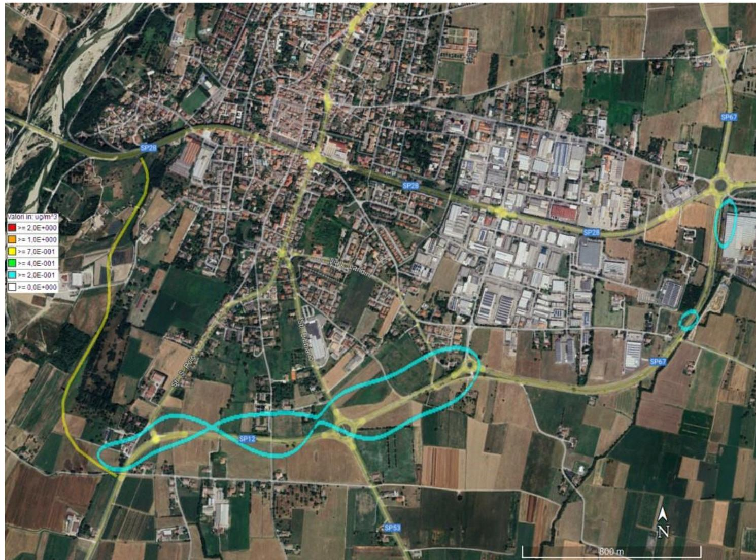
Figura 35 Concentrazione oraria al 99,8° di NO<sub>2</sub> – scenario 3 ( $\mu\text{g}/\text{m}^3$ ).
